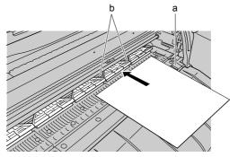
When the cut sheet is inserted, the printer grabs it and holds it on the platen.
